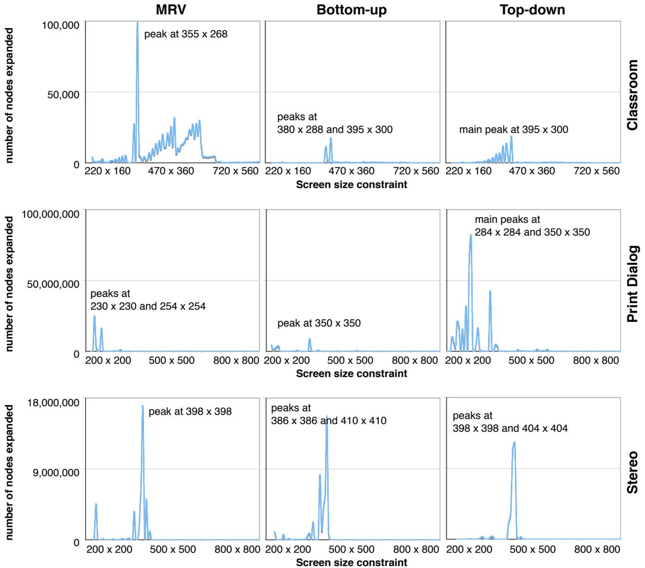
Figure 24: Algorithm performance (quantified by the number of nodes considered by the search algorithm) for three different user interfaces studied systematically over 101 size constraints for three different variable ordering heuristics: minimum remaining values (MRV), bottom-up and top-down.
