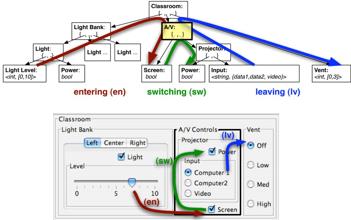
Figure 8: Three types of transitions between elements of a user interface illustrated with respect to the A/V interior node: *entering* (ent), when a descendant of A/V node is manipulated following an element that is not its descendant; *sibling switching* (sw), when user manipulates two different descendants of the A/V node; and *leaving* (lv), when a user manipulates a descendant of A/V and then navigates to an element outside of the A/V sub-tree.
